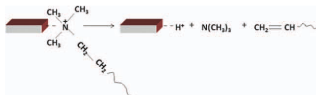
Figure 10 The mechanism of degradation in the chlorobutyl rubber nanocomposites. [Color figure can be viewed in the online issue, which is available at wileyonlinelibrary.com .]
